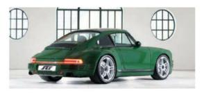
RUF Automobile's latest car, the SCR, features a RUF-designed full carbon fibre bodyshell reinforced with an integrated roll cage and monocoque chassis, is powered by a 510hp, 347lb ft, 4.0-litre normally aspirated, six-cylinder boxer engine mated to a six-speed manual transmission. Weighing in at only 1250kgs, the new SCR is a result of two years of development work, the original prototype was shown at the 2016 Geneva Motor Show.
