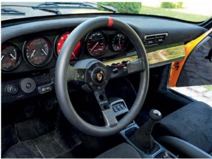
dp Motorsport utilised much of its own stock – all made out of carbon and weighing less than half that of their steel counterparts.
