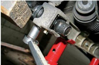
stunning and the new joints bolted straight in, complete with a new star washer and R-pin. I mentioned last month that I was able to fit all the bushes with only the standard tools in my garage. This was also true for the front bushes on the A-arms, but they did put up a fight. I was able to use a vice and press them in, but if I was going to do it all again I'd make a tool from some threaded bar to wind them in.
